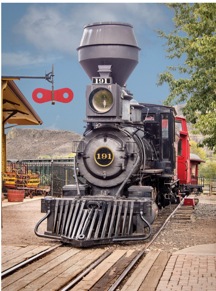
Note the dual-gauge rails beneath Denver, South Park and Pacific Railroad No. 191 , at the Colorado Railroad Museum. (Photo by Ken Boyd)
