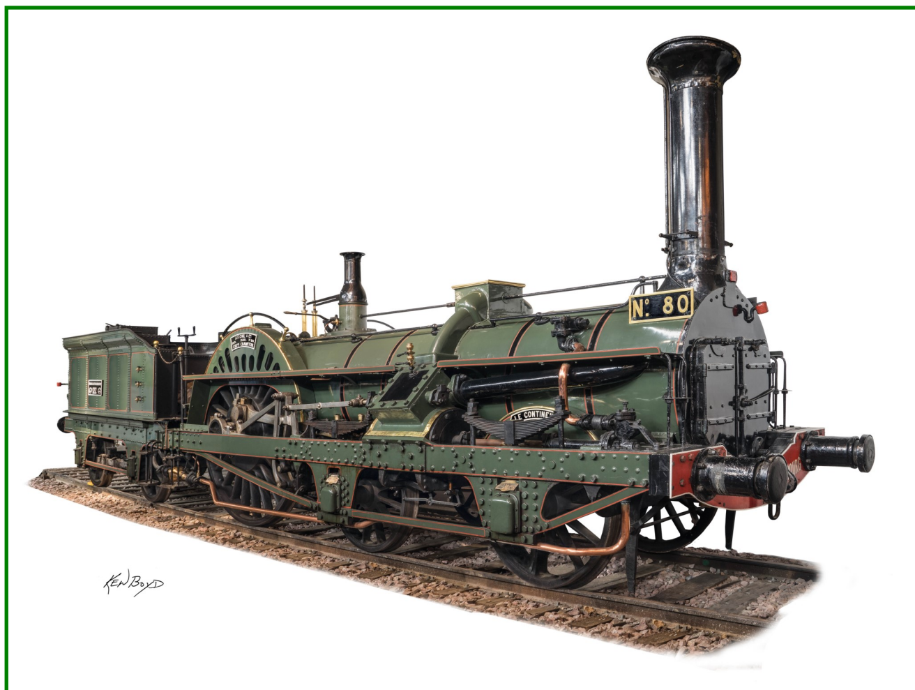
No. 80, Le Continent , 1852, at the French National Railway Museum. Note the massive double frame. The open driver platform was common in Europe through the mid-1800s. Photo by Ken Boyd.
