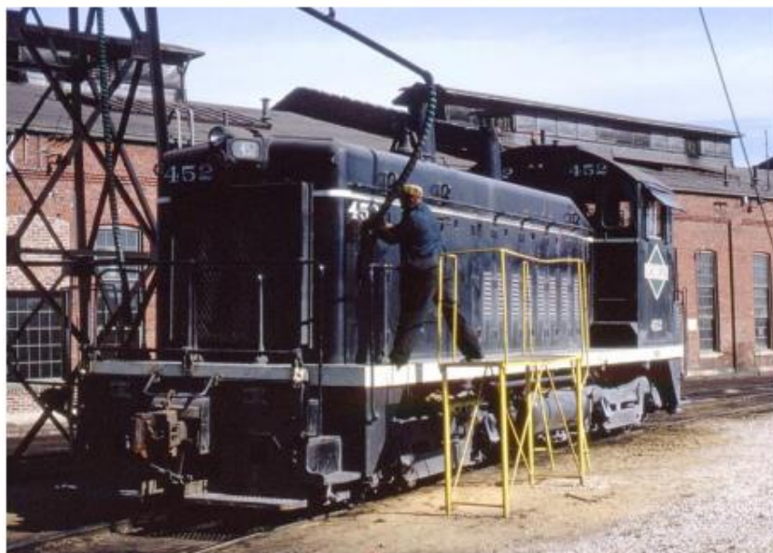
Frisco Baldwin V0-1000 215, built in 1943 and re-engined with a 12-cylinder 567C by EMD in 1959, switches on SLSF's Birmingham Belt subsidiary north of downtown.
