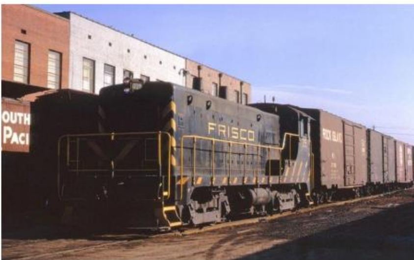
Frisco Baldwin V0-1000 215, built in 1943 and re-engined with a 12-cylinder 567C by EMD in 1959, switches on SLSF's Birmingham Belt subsidiary north of downtown.
