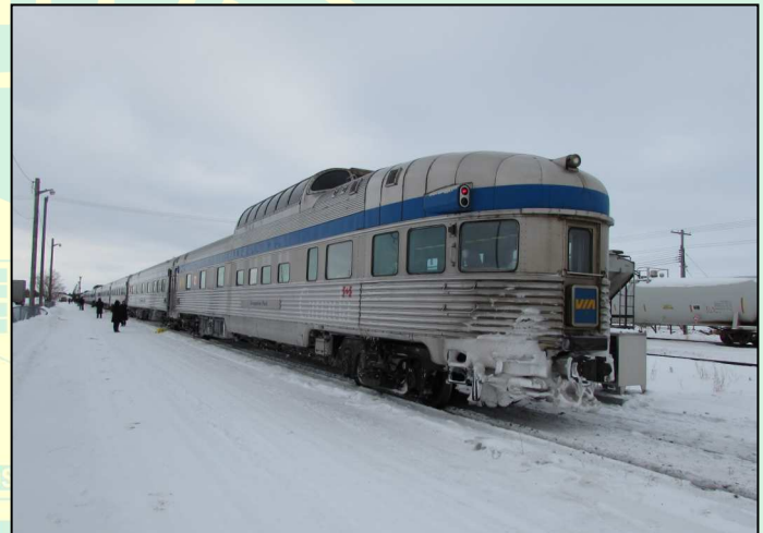
"Evangeline Park" at Saskatoon, Saskatchewan shows the ice and snow that had accumulated underneath the car's skirt.
